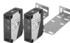
D – devices detecting the presence of persons or obstacles located on the ground on one side of the door, e.g. photocells. NOTE In case of using combination C + D, it is required that device D be checked periodically at intervals of not more than 6 months.
